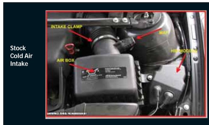
it from heat generated by the engine. The stock system is restrictive, though, making the air work its way around in order to enter the engine. After market intakes try to accomplish one primary goal: to better inject colder air directly into the intake system with fewer restrictions.
