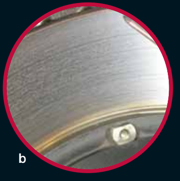
A brand new rotor before (a) and after (b) bedding in the pads. Note the even transfer layer of pad material onto the surface of the rotor, as well as the coloration of the disc itself indicating that it has been hot.
