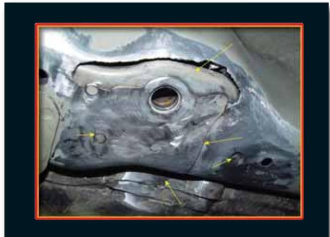
through the axle and to the wheels, force is applied to the sub-frame.
